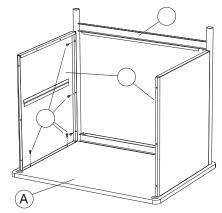
2 Slide the D Back Panel into position between the Side Panels as shown in the inset. Keep the Back Panel inside the flanges on the Side Panels. Fasten the Side Panel and Back Panel to each E Rear Leg using three L Screws from the interior.
