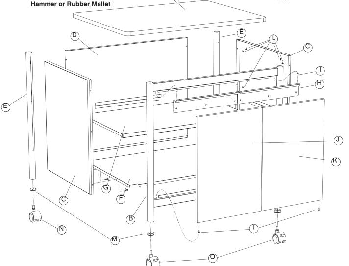
Work on a smooth, clean surface. Place the A Top Panel face down with the holes up. Position one © Side Panel on one end of the Top Panel with the flanges toward the center of the unit. Fasten the Side Panel to the Top Panel with two L Screws
