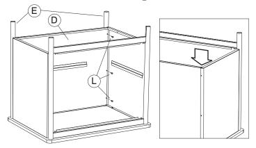
Slide the FBottom Shelf into the unit between the Side Panels, with the flanges toward the bottom end of the unit. Slide the flanges of the shelf into the lower flanges on the Side Panels
