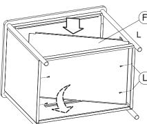
Slide the (a) Inner Shelf into the unit between the Side Panels, with the flanges toward the bottom end of the unit. Slide the flanges of the shelf into the shelf holders on the Side Panels and Back Panel.
