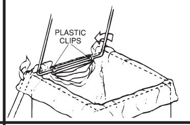
Lower wire hold-down ring into place, tuck all bag flaps neatly into inside of container (over the wire), and close the lid.
