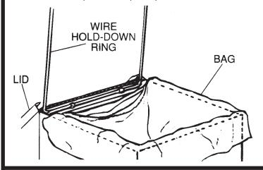
Pull two back corners of bag under corners of wire hold-down ring until bag is next to the plastic clips.
