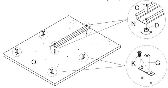
Use the Screw to connect the Legs and the Frame (A) to the Top (O). Use the Screw (K) to connect the Metal Plate (E) with the Top (O);
