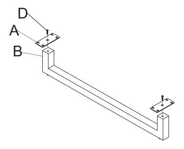
Use Screw (E) to connect the U Shape Base (B) and the Bracket (A) to the bottom of the Pedestal.
