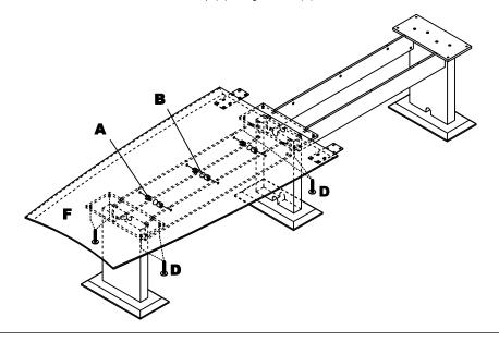
Place other Top (F) onto Legs, Center Base and Modesty Panel and lock in place by turning Cams (A). Attach the Top to the other Top using Screws (E). Apply Cam Stickers (B) onto Cams (A) of Modesty Panel. Install the STECAB Center Base to the underside of Top (F) using Screws (D).
