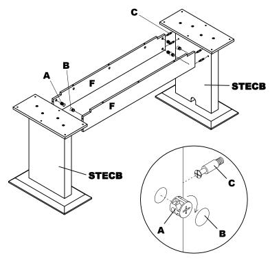
NOTE: The arrow on the face of the Cam (A) should point towards the Cam Post (C) for proper alignment.
