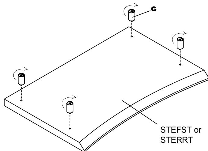
**3** Install the STECC to the underside of STEFST or STERRT Top using Screws (D).
