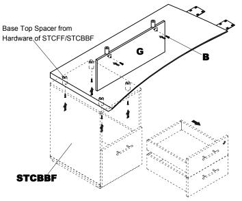
Attach Mounting Plates to the underside of adjacent Main Desk using Screws and Wrench (C).
