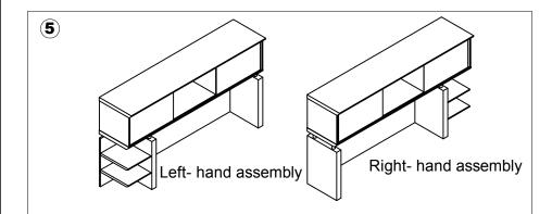
Place hutch 72"/66" and support frame 72"/66" onto Credenza 72" STCT72/66 and STECT72. using L Mounting Plate (E) ,Screw(G) and screw (F).
