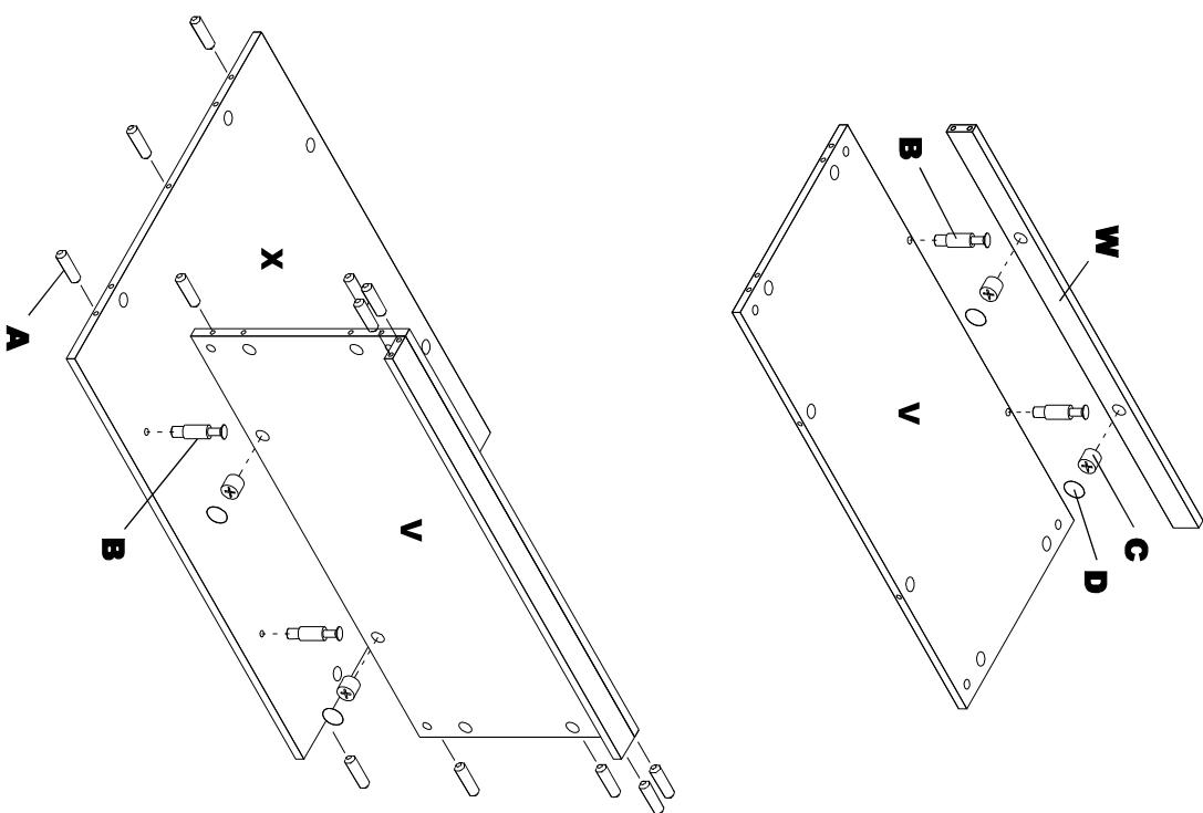
Note: For Step 2, dowels (A) are to be inserted into panels (X/V) and NOT in panels (Y1/Y2/Z) in step 3.
