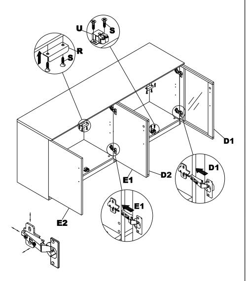
Note: Adjust door alignment as necessary by using the adjustment screws on the hinges.
