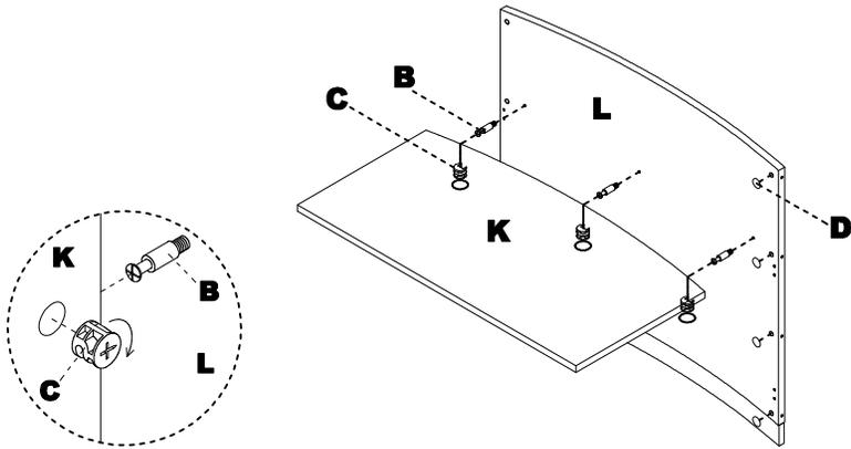
NOTE: The arrow on the face of the Cam (C) should point towards the Cam Post (B) for proper alignment.
