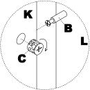
NOTE: The arrow on the face of the Cam (C) should point towards the Cam Post (B) for proper alignment.
