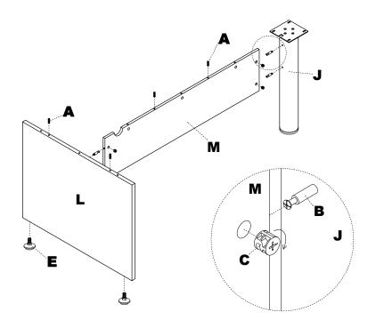
NOTE: The arrow on the face of the Cam (C) should point towards the Cam Post (B) for proper alignment.
