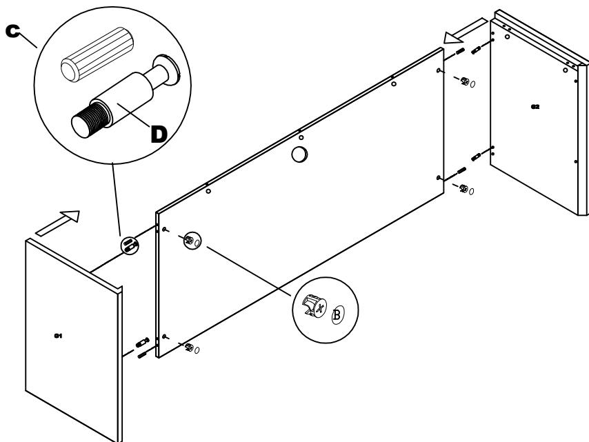
Note: For Step 1, dowels (C) are to be inserted into modesty panel (I) and not legs(G1/G2).
