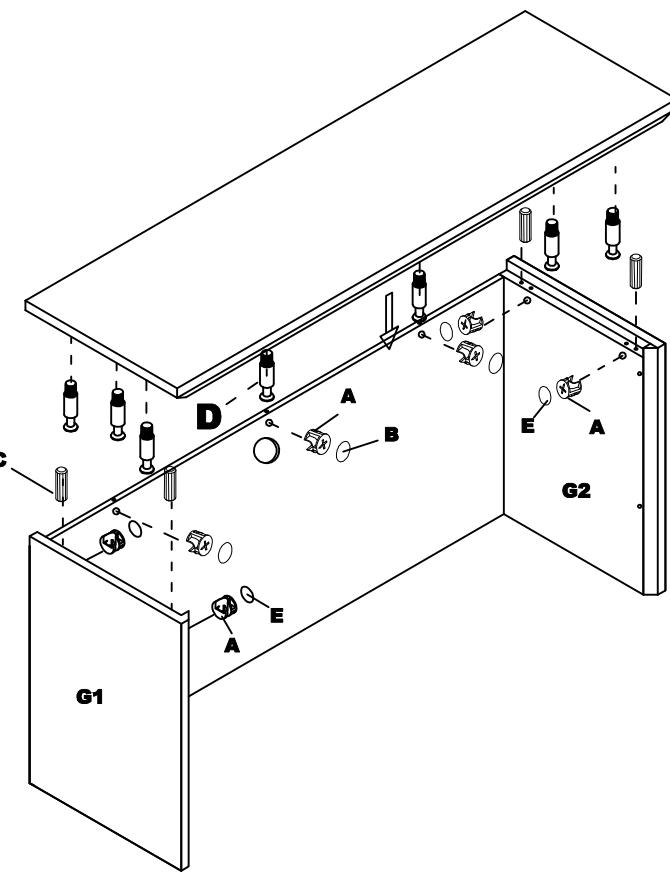
Note: For Step 2, dowels (C) are to be inserted into legs (G1/G2) and not into top (H).
