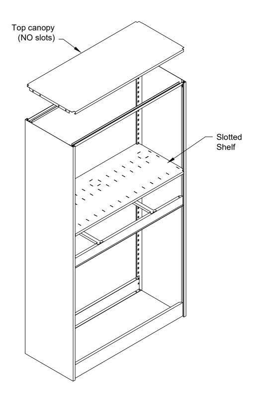
36" SHELVES: The four post units with drawers will use a shelf that has slots for the back stop and dividers arranged for both letter and legal media. The top canopy will not be slotted.
