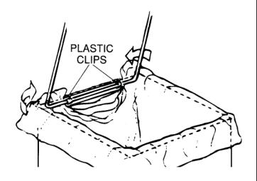
6 Lower wire hold-down ring into place, tuck all bag flaps neatly into inside of container (over the wire), and close the lid.
