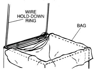
Pull two back corners of bag under corners of wire hold-down ring until bag is next to the plastic clips.
