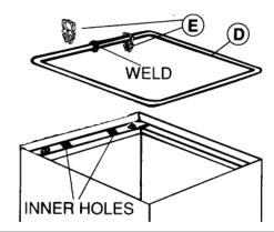
Insert © Plastic Tray into bottom of container to catch occasional drips or leaks.
