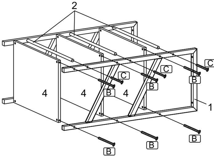
DO NOT TIGHTEN THE SCREWS BEFORE ALL SCREWS ARE IN PLACE
