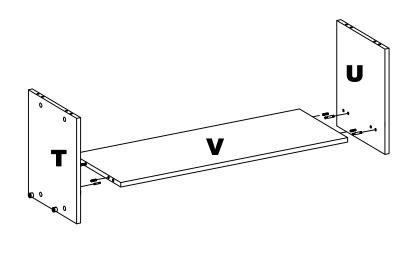
Install Cam Posts (B) into threaded inserts in Shelf (M) and Center Shelf (V). Insert Wood Dowels (A) and Cams (C) into Left and Right Dividers (T, U) and Paper Dividers (W). Secure boards by locking Cams (C).
