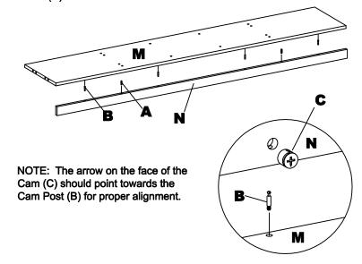
Install Cam Posts (B) into the threaded inserts in Back Panel (P). Insert Wood Dowels (A) and Cams (C) into Shelf (M). Secure boards by locking Cams (C).
