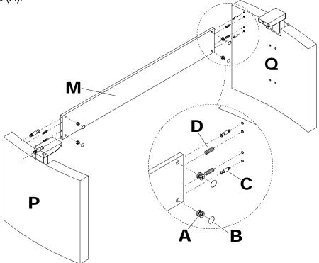
Place Top (K) upside down on a clean non-abrasive surface. Insert Wood Dowels (D) and Cam Locks (A) into the Modesty Panel (L). Install Cam Posts (C) into the Top (K). Attach Modesty Panel (L) to top by turning Cam Locks (A). Attach Stickers (B) over Cam Locks (A).
