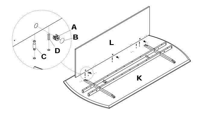
Install the Control Box (S) to Top (K) using Screws (R). Install the Bracket (I) to the Modesty Panel (L) and Top (K) using screws (E).
