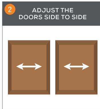
Slightly turn the **adjusting screw (D)** on **both** hinges on each door. **You may have to slightly release the locking screw C to do this.** Make sure it's tight afterwards
