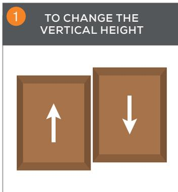
Undo the two **adjustable cupboard screws (B)** on both hinges. They are usually in slotted holes, which means you can adjust up or down by a few mm, then tighten back up.
