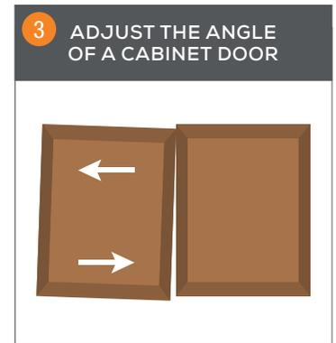
Use the **adjusting screw (D)** but this time only screw either the top or bottom screw. For a bigger adjustment, screw the top one way and the bottom the other! You may need to slightly release the **locking screw (C)** to do this. **Make sure it's tight afterwards.**
