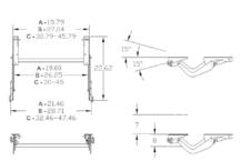
Sit/Stand height-adjustable keyboard arm with paddle actuated spring brake height adjustment and lever for tilt. Variable width configurations, fixed mount application. Available in 19", 26.25" widths.
